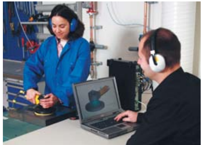
Atlas Copco has a well equipped laboratory for measuring tool noise and vibration emissions. It contains advanced vibration measurement tools, a state-of-the-art acoustics laboratory and dedicated computer software for analysing measurement and test results.
