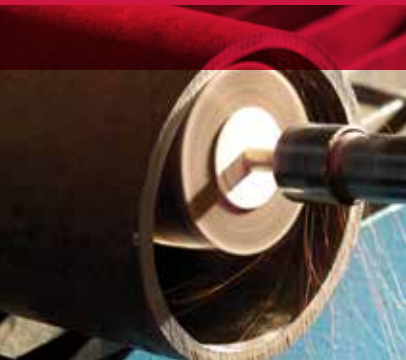
Removing burrs from the inside diameter (ID) of a cut tube.
