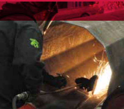
Weld removal with Tiger combo wheel.
