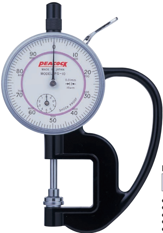
PG-10 Graduation: 0.01mm Range: 0~10mm ● Throat Depth 20mm ● Accuracy \pm 20\mu m ● Contact Point dia. 10mm ● Parallelism 5\mu m ● Measuring force less than 1.8N
