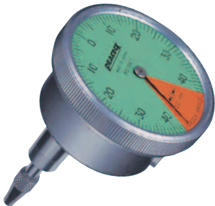
196Z Graduation: 0.01mm Range: 0.8mm ● Stem \phi 8mm ● Pointer giving less than one revolution ● Contact point (X-112)
