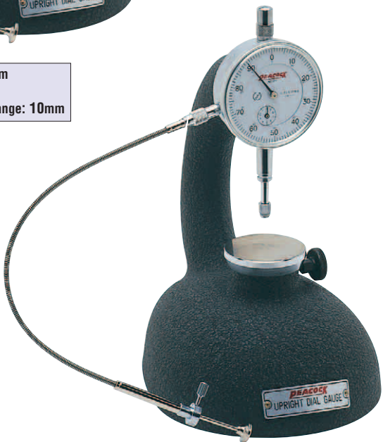
R1-B Graduation: 0.01mm Range: 10mm Effective measuring range: 25mm
