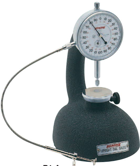
R1-A Graduation: 0.001mm Range: 2mm Effective measuring range: 10mm
